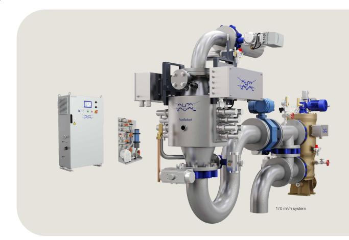
Now in its third generation, Alfa Laval PureBallast is an automated inline treatment solution for the biological disinfection of ballast water. Operating without chemicals, it combines initial filtration with an enhanced form of UV treatment to remove organisms in accordance with stipulated limits.
