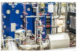
Soft drink mixer with Alfa Laval M10 and M6 heat exchangers and SolidC pump.
