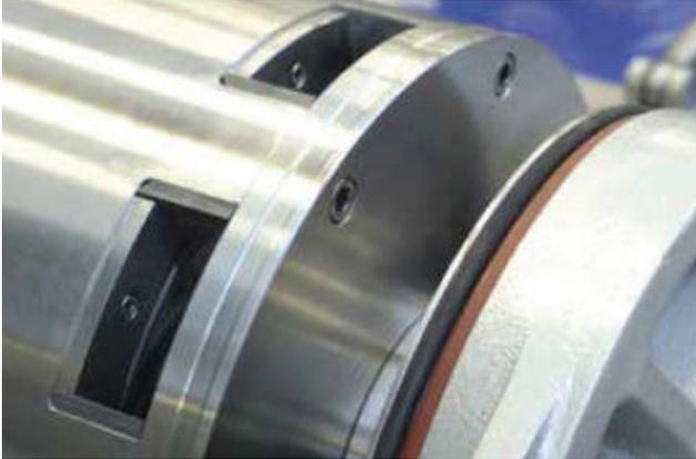
Figure 3. Solids discharge, free from blocking
