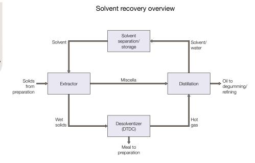
The solids are typically processed in a unit called the desolventizer (DTDC), whose main function is to flash the volatile solvent from the solid phase by use of direct steam injection. The vapour leaving the DTDC must be cleansed and condensed.
