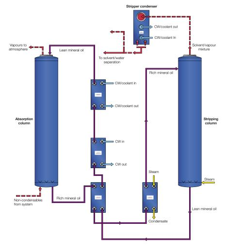
Example flow diagram - Vapour scrubbing
