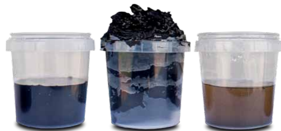
Mill effluent (left) before dewatering in a decanter. This separates it into 10% cake (middle), which can be used as fertilizer, and 90% liquid centrate (right), that can be further polished to meet final effluent discharge parameters.
