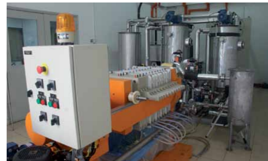
Alfa Laval's dry fractionation pilot plant in Malaysia is used to customize a solution to suit customer requirements to different types of feedstock, and for R&D.
